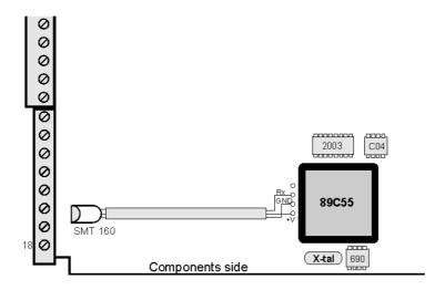
Cold Junction compensating sensor SMT 160 is glowed at the cabinet rear side near to the screw terminals.
