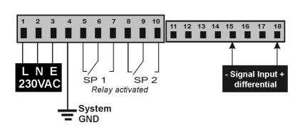
Input 18 (+), 15 (-) differential Configuration R31 = shorted H1 = 1H3 = 1 for DC, H3 = 2 for RMS Set in =  $0.0 \ 1$ Range **R34** Range **R34** 20mV 511r 150mV 3k92 50mV 1k3 200mV 5k62 100mV 2k67 250mV 6k98
